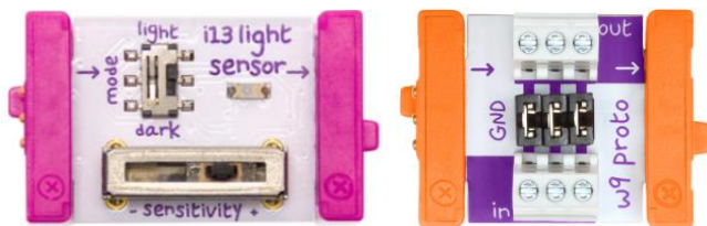
Fig. 7. Receiver components: Light sensor and proto bits.
